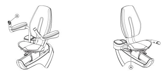
At-Your-Fingertips Resistance Controls are located on the right armrest and right side handlebar on the Recumbent Lifecycle Exercise Bike.
